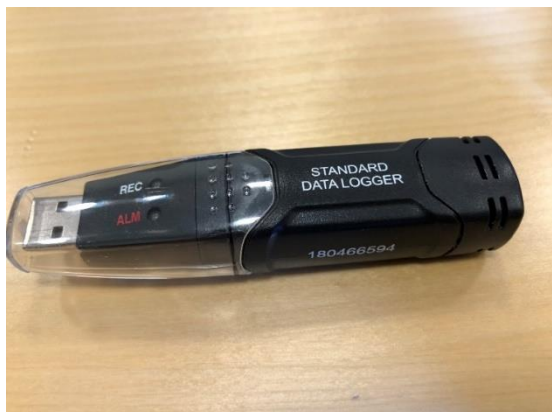
Figur 42. Fuktlogger Standard ST-171 datalogger.
